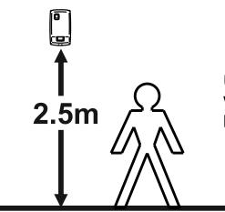
Using the fixings provided secure the backplate to the wall at 2.5 metres above the floor. To obtain optimum performance do not site the unit close to air extraction.
